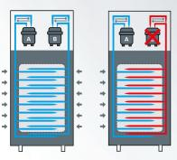
In case of a failure, the TRUE DUAL<sup>™</sup> technology maintains a stable temperature of +4 °C and protects the blood.
