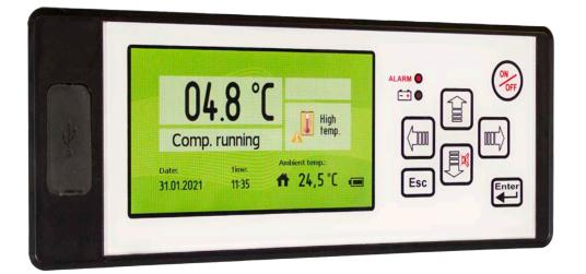
The G214 controller is used on most of our units. It has been ARCTIKO's main controller for many years. With regular updates, the G214 controller has stayed ahead of the competition. The controller has all the features needed for safe storage of your valuable samples.
