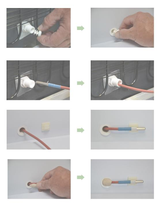
Never install probes through the door as this will deterior the functionality of the door gasket and the temperature inside the unit.
